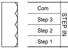
Used when connecting a gyro compass with stepper output.
