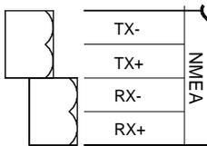
NMEA signals from compass or speed log with serial output should be connected to RX- and RX+. Refer Dip switch settings for speed, page 4.
