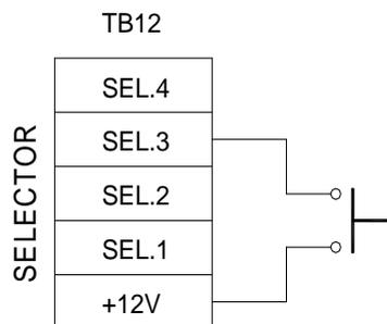
The switch must be a potential free pulse type. When pressing and holding the switch, the heading will increase or decrease, depending of last direction control.
