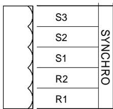
Used for connecting gyro compasses with synchro output. Refer *Dip switch settings*, page 4 for signal specification.
