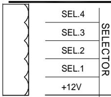
The selector lines option on TB12 are used both for heading offset adjustment and for the optional pendulum function key as described below.
