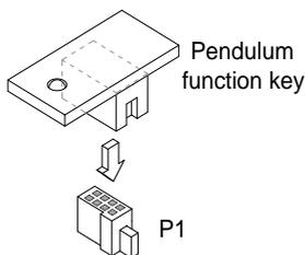
3. Carefully insert the pendulum function key into P1. Observe the guiding slot as indicated on the figure.
