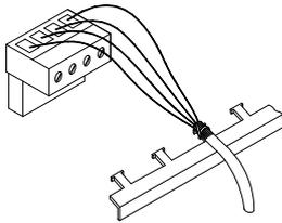
To make a good ground connection, strip about 1 cm (0.4”) off the cable’s insulation and pull the screen backwards to cover the insulation. Position the straps as shown in the figure. Tighten well to make sure the screen makes good contact.
