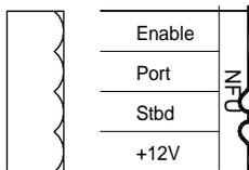
Used for connecting a remote Non Follow Up lever. Rudder command or course change will be sent to the autopilot via Robnet.
